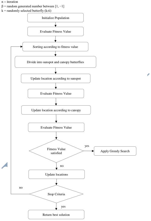
Figure 2: Algorithm for Artificial Butterfly Optimization
