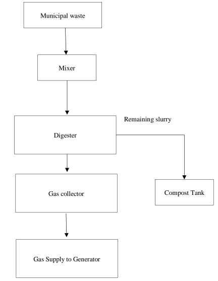
Figure 1: Flow chart of biogas production system
